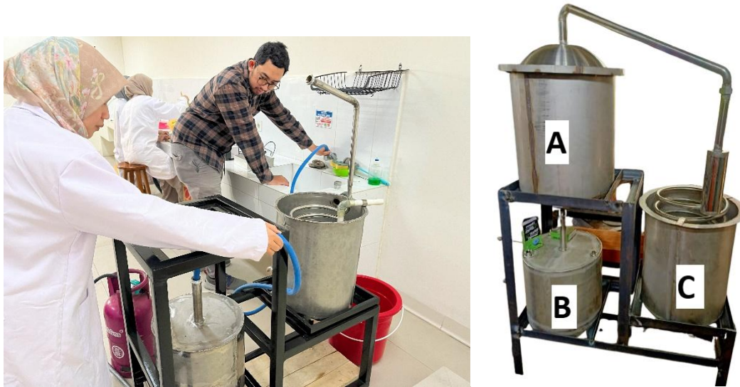
Figure 8. Documentation of the distillation apparatus trial (left); Appearance of the distillation apparatus (right)
