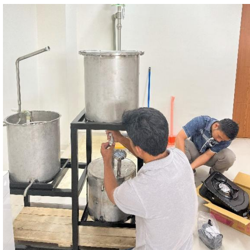
Figure 7. Assembly of essential oil distillation equipment by supplier
